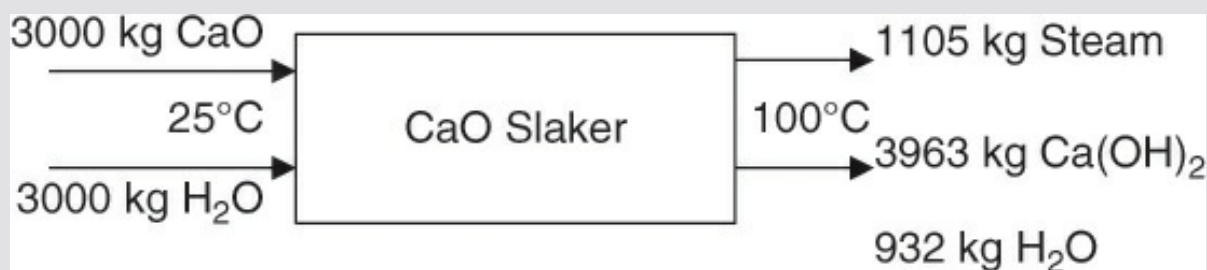
Figure 7.8 Material and energy balance on a CaO slaking operation.
